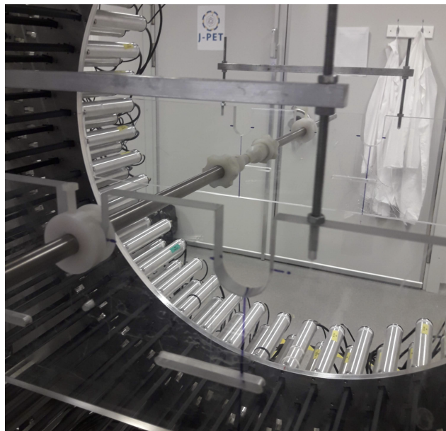
(c) Annihilation chamber (fig. 4.1) placed in the center of the detector. This chamber was attached to two metal rods which were then placed on a movable plastic holders. Such setup allowed to fine-tune the position of the source to be in the center of the detector.
